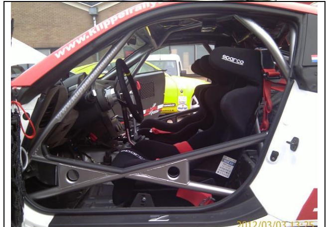
PHOTO 10 DRIVER'S DOOR ANTI-INTRUSION DOORBAR
